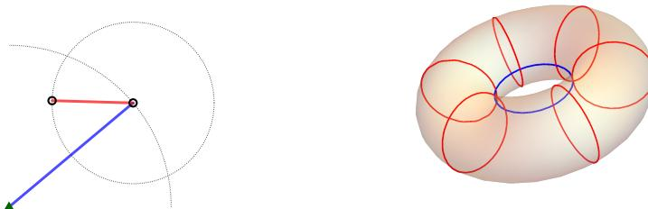
Fig. 2: (left) 2-R planar mechanism. The blue arm revolves about the fixed point, while the red arm is connected with a revolute joint to the second endpoint of the blue arm. (right) The configuration space of the 2-R planar mechanism. The blue and red circles represent the respective rotations of the arms.
